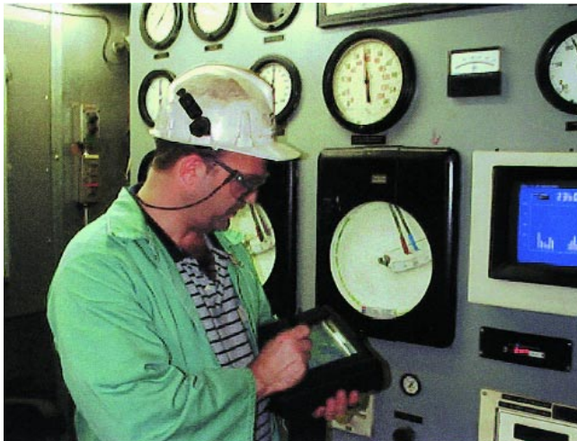
Fig. 3 — View of an operator using a handheld data logger to capture data about an asset for analysis in the ICMS system.
